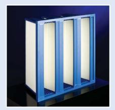
The filter packs are completely sealed in the plastic casing made of pure polymer, therefore the filter can be extremely high mechanically charged. The burst pressure drop of this construction is far above 3000 Pa.
