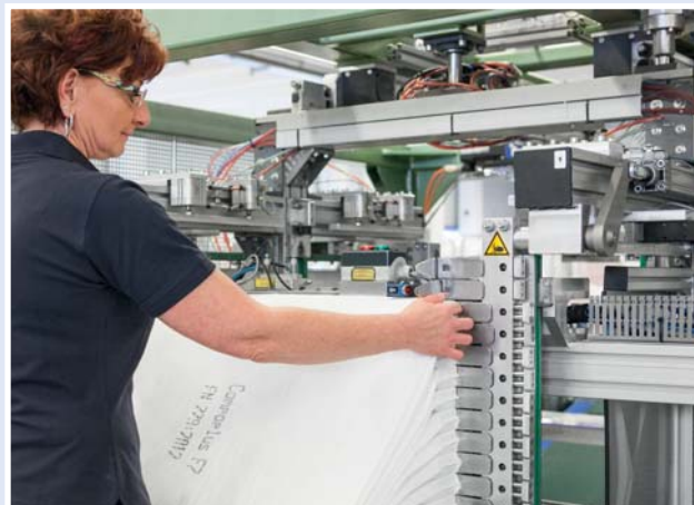
Compoplus® pocket filter welding unit
