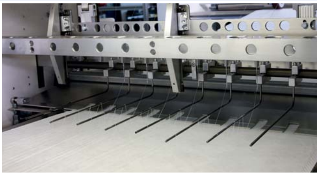
Compoplus® pocket filter stitching unit
