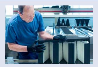
As a result of the pleating, a comparatively large filter area with high stability results, which opens up special fields of application to compact filters. In particular, this construction design is used where high nominal airflow rates, large stability and high separation capacity are involved, for example in gas turbines, off-shore plants or for the protection of high-quality applications in cleanroom technology.
